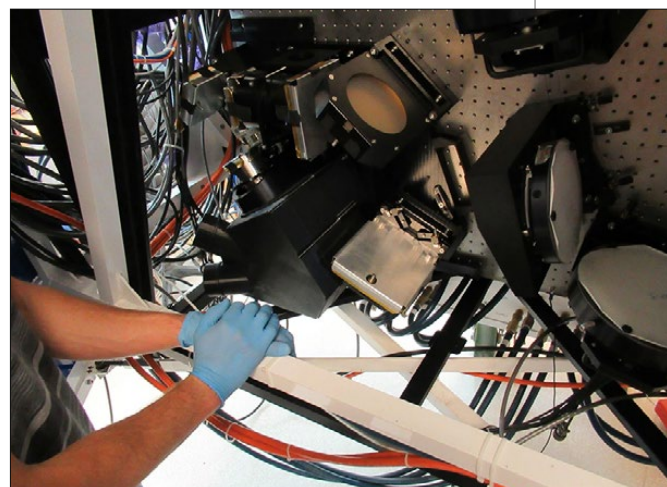
Figure 4. The new NGS2 unit after installation into the Canopus optical bench.
